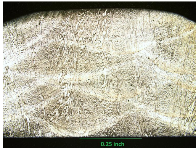
Figure 5.42 Macrostructure of ENiCrMo-4 mix 7
