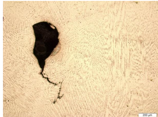
Figure 5.47 ENiMo-10 slag inclusion and crack
